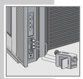
1 Connect the yellow socket (VIDEO – picture signal) on the television and the corresponding socket on the camcorder (VHS, Video 8) with a cinch cable;
